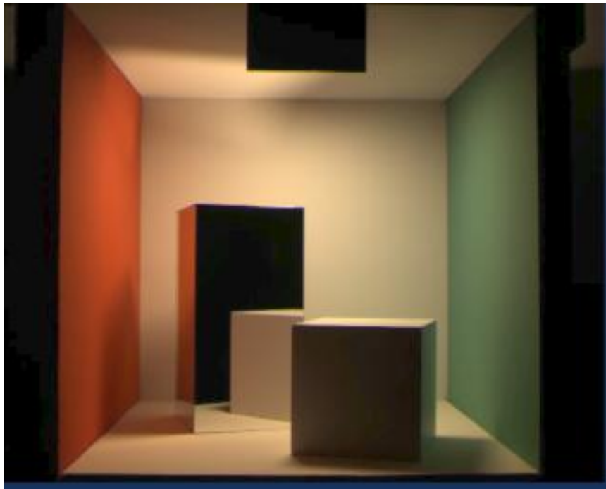
Measured radiosity (CCD image)
